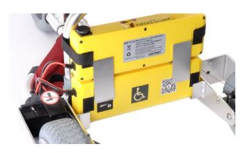
3. Place the second (upper) battery into the Hbrackets and align with the lower battery. The upper battery wire should be in the lower left corner (viewed from the rear) to allow for connection to the TravelScoot without rearranging the battery positions.
