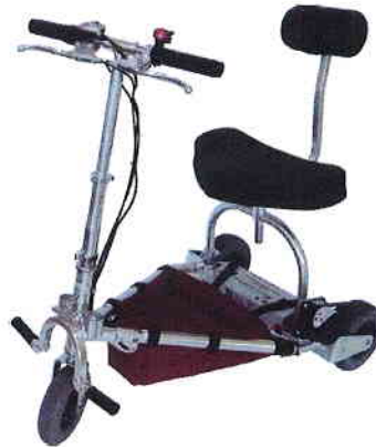
Figure 4.2 – Collapsible lithium battery powered mobility aid
